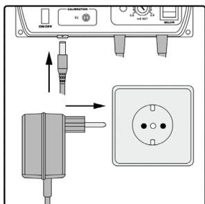
Connect the supplied 240VAC/12VDC power adapter to the meter and to the main line.
