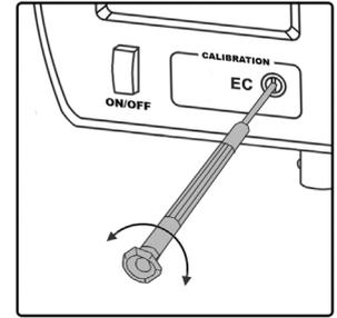
The calibration is now complete and the meter is ready for use. The instrument should be re-calibrated at least once a month, or when the probe is changed.
