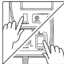
A blinking alarm will indicate when the measured pH value is higher or lower than selected setpoint, depending on user selection. When the alarm is activated, it also activates the connection base and the auxiliary equipment.
