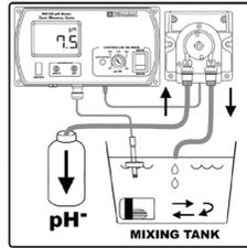
Connect the pump to the MC122 pH controller (on the black and white outlet). The pump will discharge 0,08 cL every 2 seconds.
